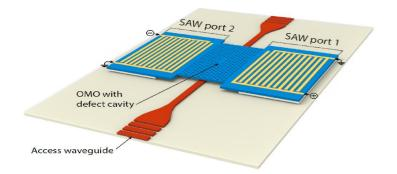
Schematics of the fully-integrated optomechanical platform integrating the photonic crystal optomechanical oscillator - OMO - (in blue - allowing for an optical control of mechanical motion), an integrated optical waveguide below the resonator (in red) and surface acoustic wave transducers on top (in yellow allowing for an acoustical control of mechanical motion).
