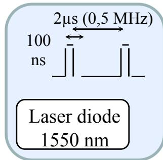
CW laser modulation @ pulsed laser frequency (500KHz)
