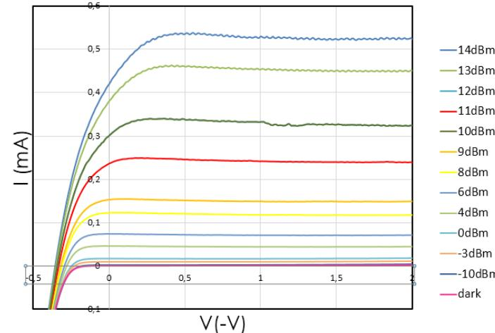
**Shot-noise** measurement to be able to evaluate **excess noise** from the channel (CW optical input)
